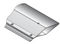
Both blade material options have interlocking engagement to provide low leakage and optimum fire resistance when closed.
